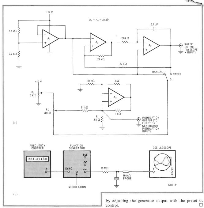
**Small scan.** Low-level modulator (a) superimposes small fraction of 10-V triangle wave on preset dc voltage so that externally driven function generator can be swept over very narrow ranges not normally within the resolving power of unit's front panel controls. In typical application (b), response of crystal and isolation of its resonant and antiresonant frequencies are displayed and recorded.
